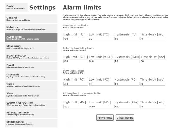
Example of setting the limit to the upper alarm limit:
